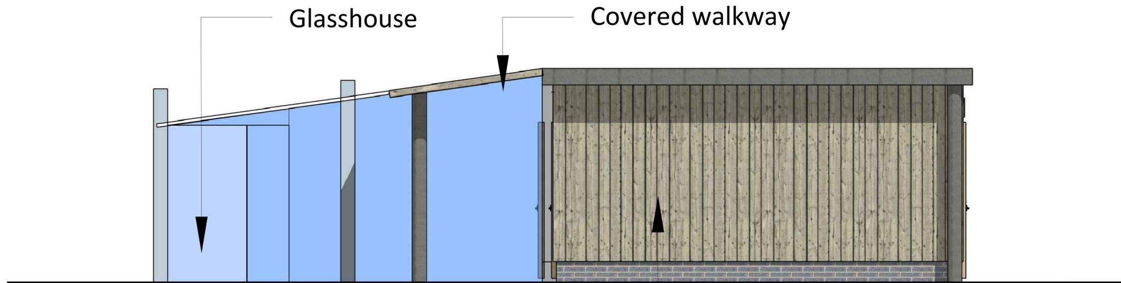
Timber cladding over concrete blockwork to exterior walls
